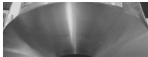
Clean Sheave Plates
