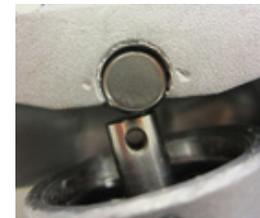
Improper Piston Alignment
