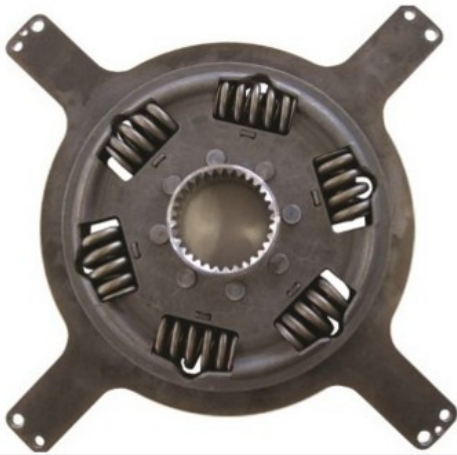
Torsional damper with a multi-stage damping effect
