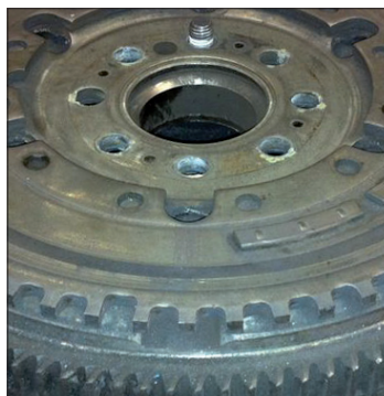
Image 1: Previous sensor ring design
