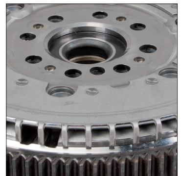
Image 2: New sensor ring design
