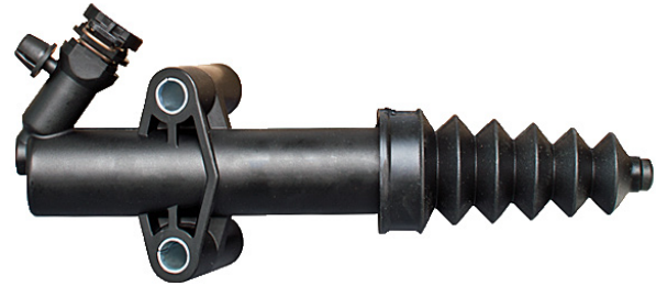
Image 1: Clutch slave cylinder 512 0050 10 (Version 1/original equipment)
