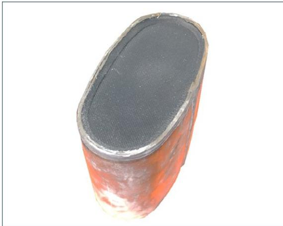
**Fig. 1** - example of stuck DPF from AUDI A3 2.0 TDI (8P model)
