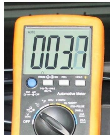
Resistance of heater circuit
