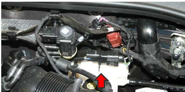
The sensor itself has 5 wires and the vehicle harness has 6.
