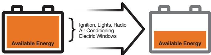
The more accessories that are in use, the faster available battery energy is consumed. Consumption of the battery's capacity is referred to as 'discharging'.
