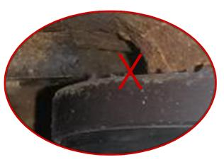
SOLUTION: The ABS sensor is being forced away from it's correct position by the rust build up behind it on the dust cover plate.
